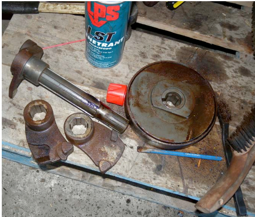
25 MAY 2010: Removed the breech block from the HI breech ring. Note the welded firing pin cover.
