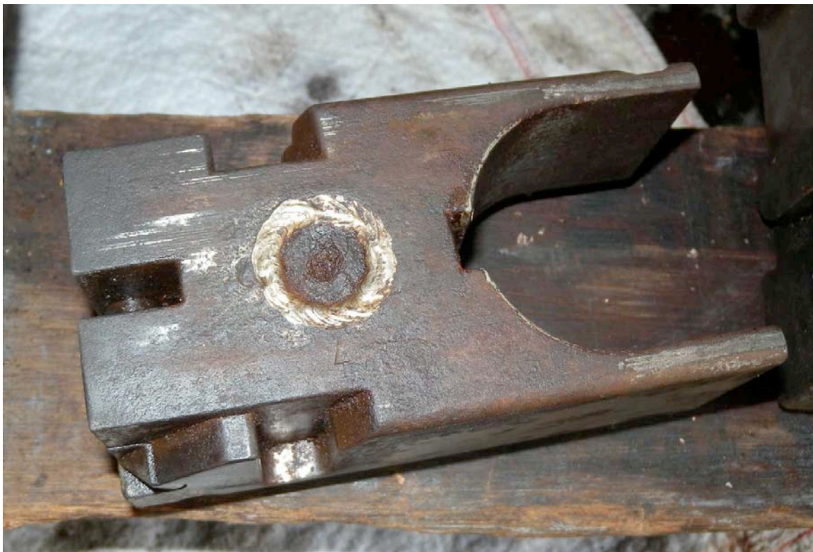
25 MAY 2010: Removed the breech block from the HI breech ring. Note the welded firing pin cover.
