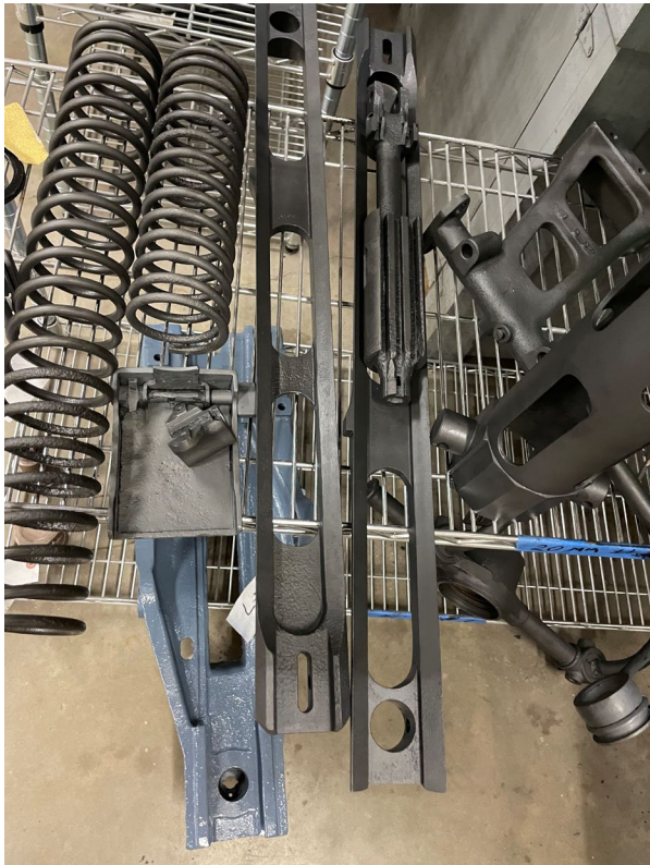
Representative barrel springs, breech bars, breech block, and trigger case cover after parkerization
