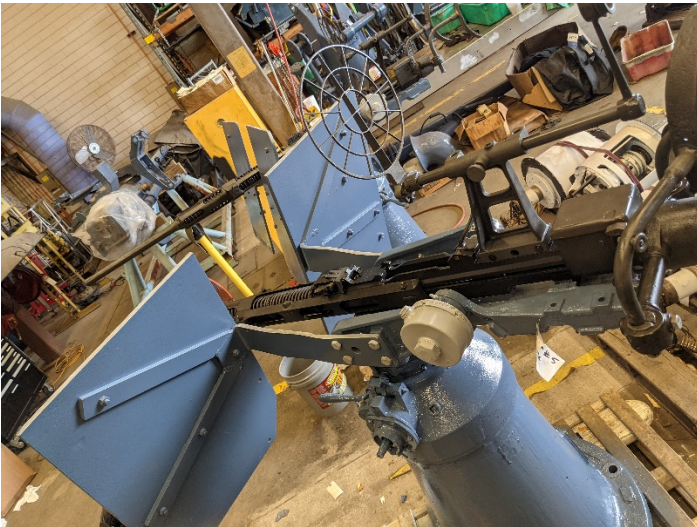
Representative mount after being reassembled with gun parkerized, prior to gun being painted
