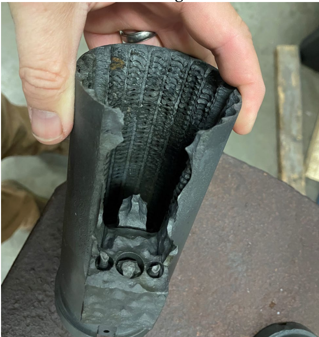
Representative trigger casing after electrolysis. The interior of the casing is almost entirely corroded away, revealing the corrosion damaged springs.
