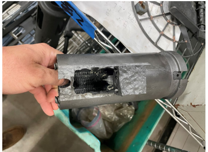
Representative trigger casing after parkerization
