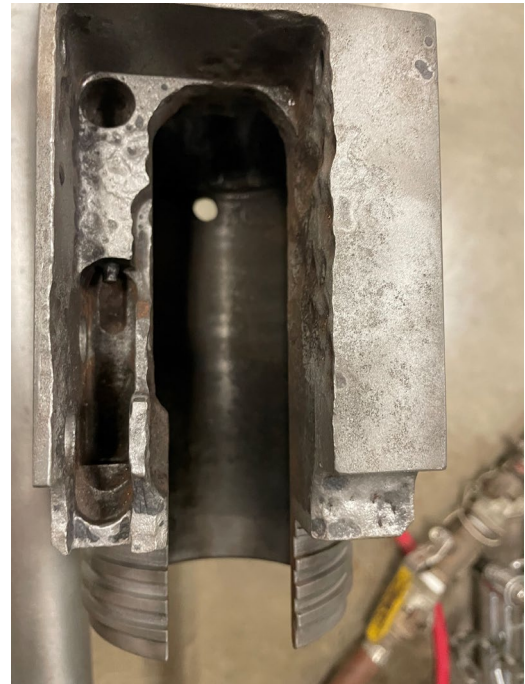
Breech casing after treatment, prior to final preparation for parkerization
