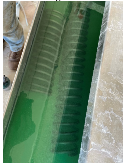
Barrel springs undergoing parkerization.
