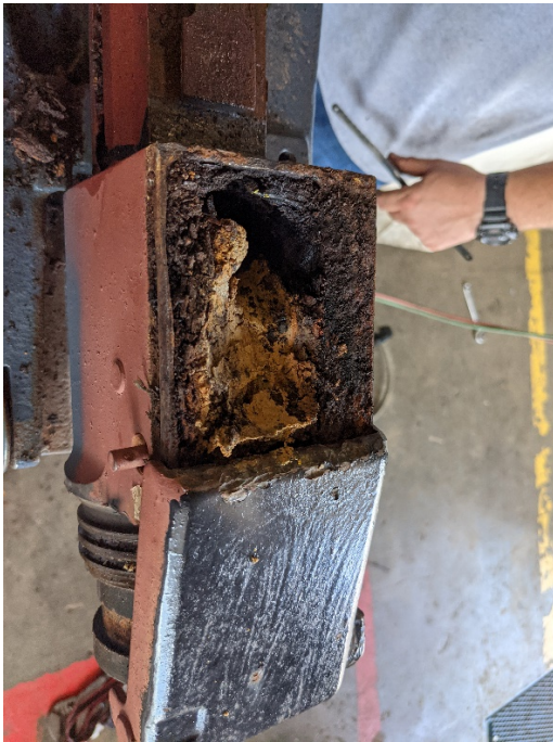
Corrosion filled interior of trigger casing/breech casing
