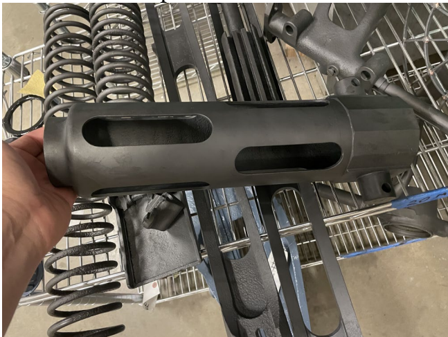
Representative barrel spring casing after parkerization
