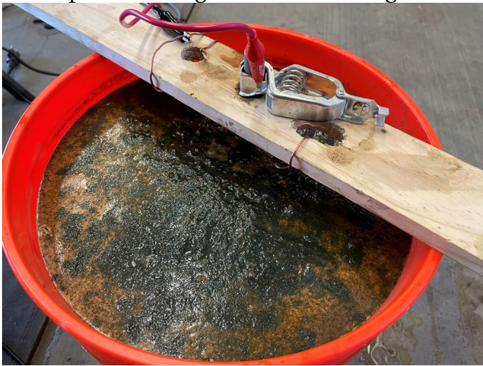
Trigger casing undergoing electrolysis. The film floating on top is rust.
