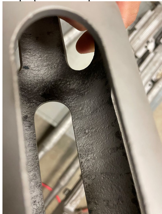
Representative barrel spring casing after electrolysis and bead blasting. Note the heavy pitting in the interior surface.
