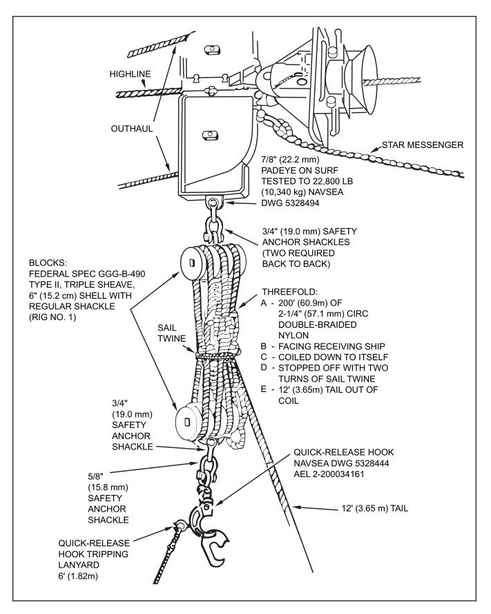
Figure 6-34. Heavy Load Return Using Threefold — Rigging at Delivery Station
