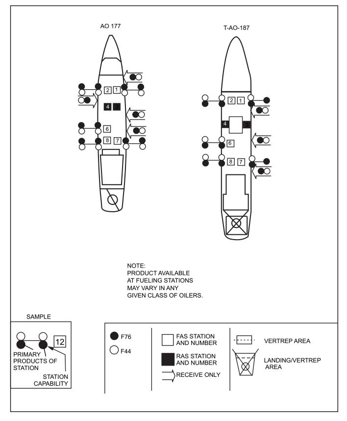
Figure 3-2. Typical Transfer Stations on Oilers (Sheet 2 of 2)
