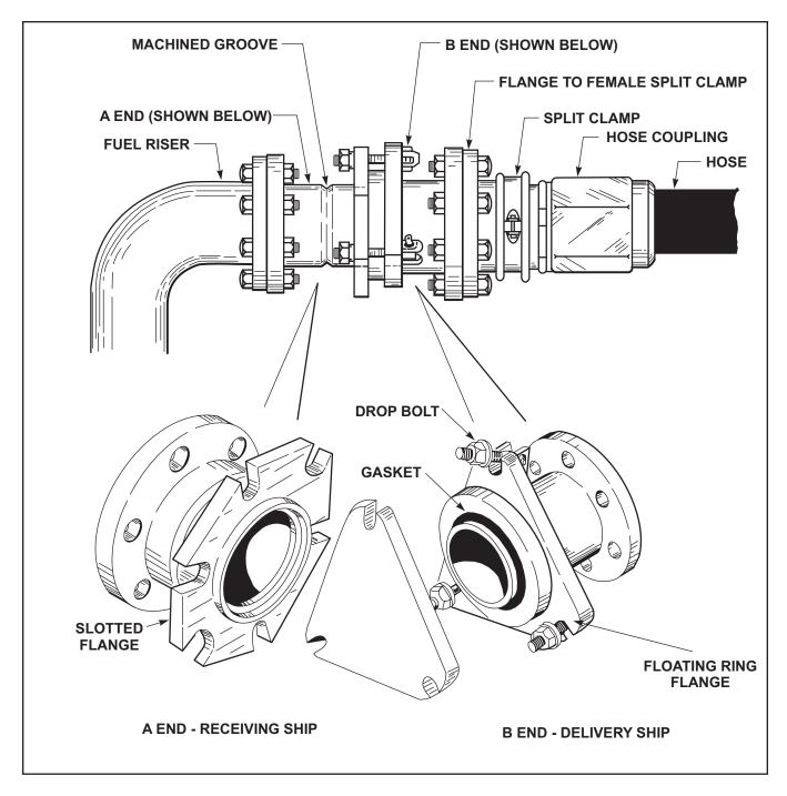
Figure 3-12. Breakable-Spool, NATO Quick-Release Coupling
