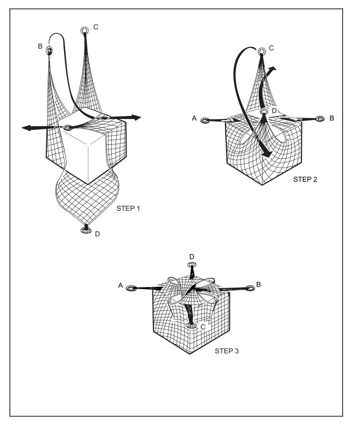
Figure 10-13. Securing Cargo Net With Loose Cargo
