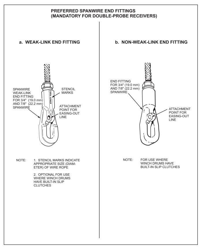
Figure 3-14. Spanwire End Fittings for Fueling Rigs (Sheet 1 of 2)
