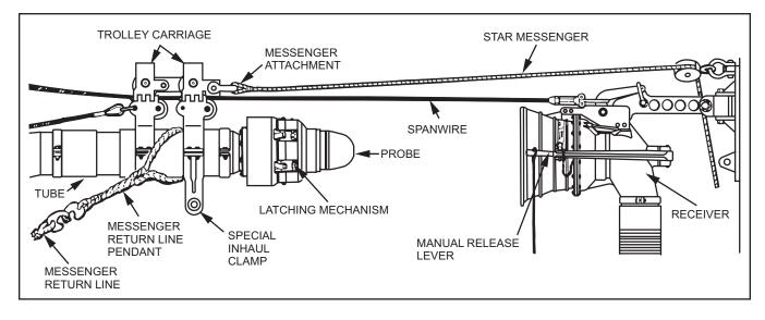
Figure 3-5. Single Probe and Receiver
