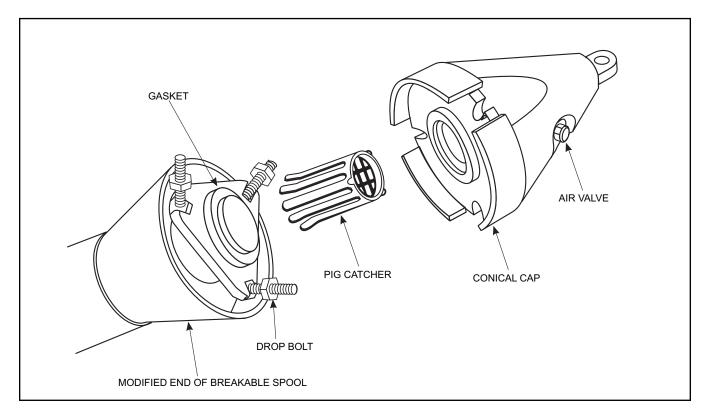
Figure 5-6. Hose End (Outboard) Conical Cap Assembly
