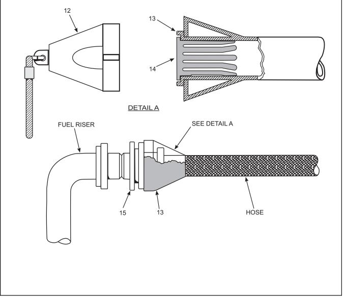
Figure J-4. Astern Refueling Station — Receiving Ship
