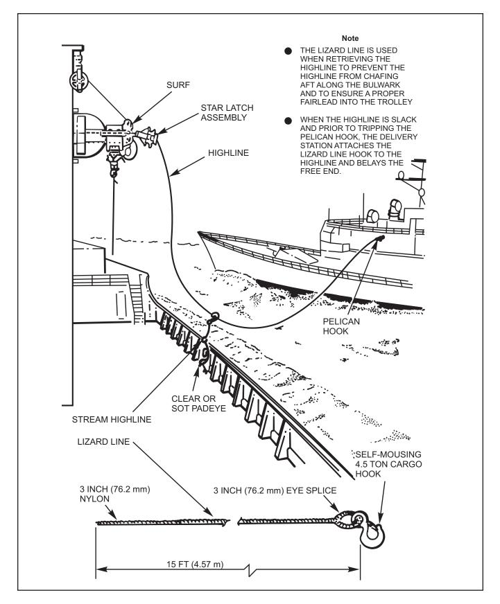
Figure 2-22. STREAM Highline Lizard Line
