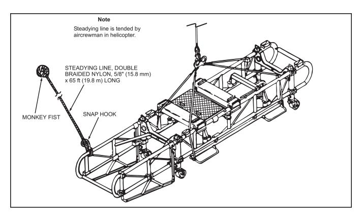
Figure 10-17. Rigging for Missile Transfer to a Class 5 VERTREP Area (FFG-7 Class Ship)
