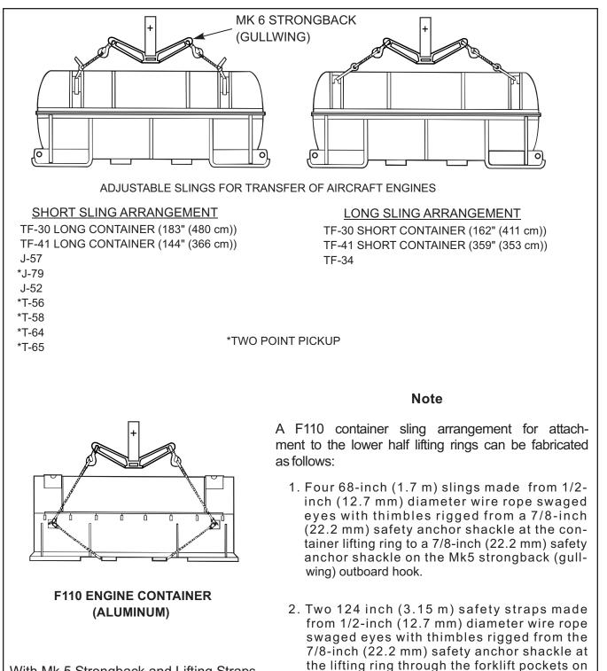
With Mk 5 Strongback and Lifting Straps Through Forklift Pockets (Safety Straps are Slack) (see Note)
