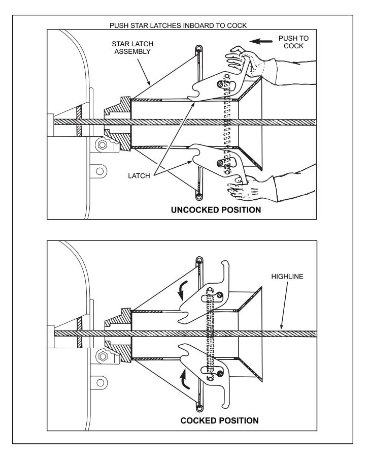
Figure 6-18. STREAM With STAR — Cocking the Latches
