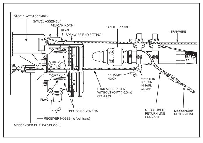
Figure 3-10. Delivering Single Probe to Double-Probe Receivers
