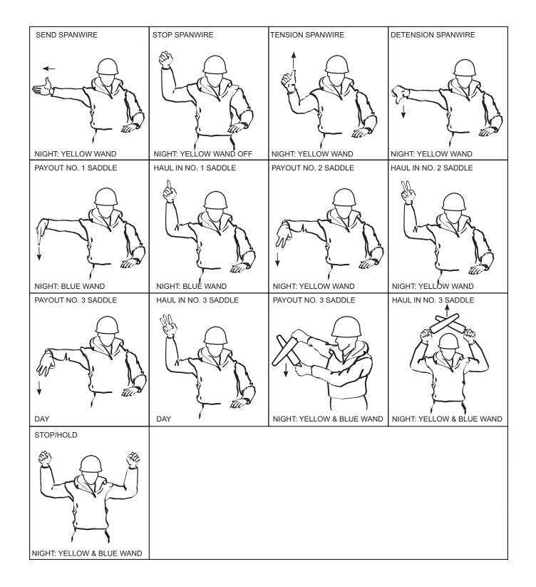
Figure G-2. Standard Hand Signals From Rig Captain to Winch Operator for Fuel Delivery Station
