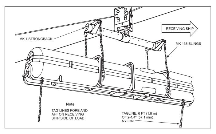
Figure 6-11. Mk 1 Strongback With Mk 183 (ASROC) Container
