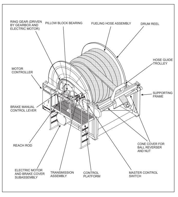
Figure 5-3. Astern Refueling Hose Reel Assembly (View A)
