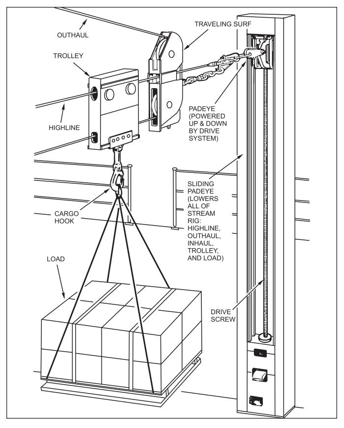
Figure 6-25. Sliding-Padeye Receiving Station — Receiving the Load
