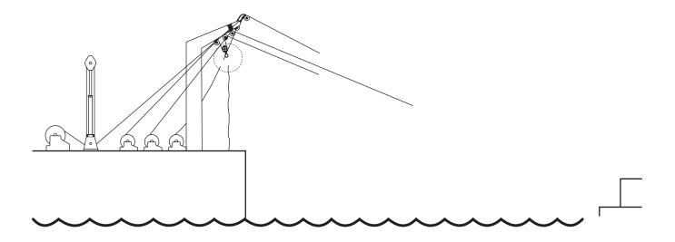
Figure 3-18. Fuel STREAM Rig - Single Hose with Probe
