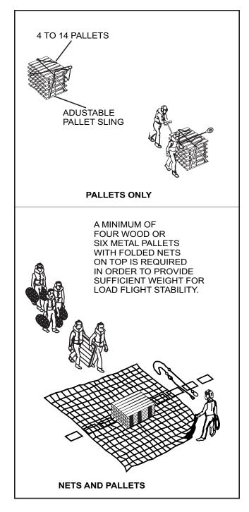
Figure 10-20. Preparation of Nets and Pallets for Return to UNREP Ship
