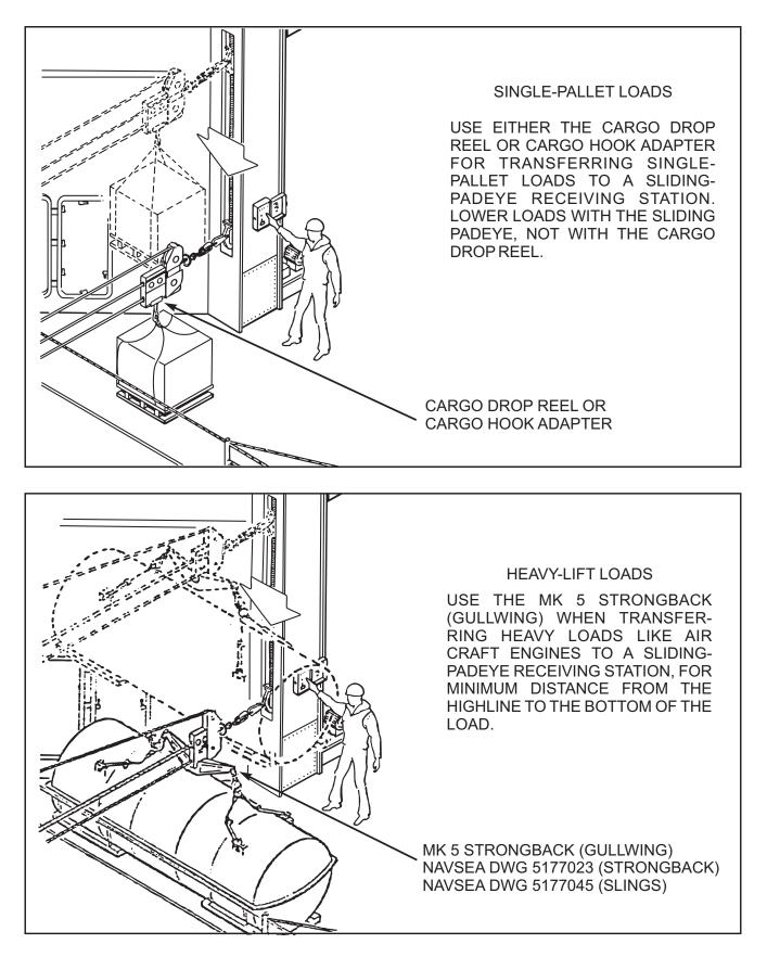
Figure 6-12. Sliding-Padeye Receiving Station (Typical) — Shown With STREAM With Traveling SURF (Sheet 1 of 2)
