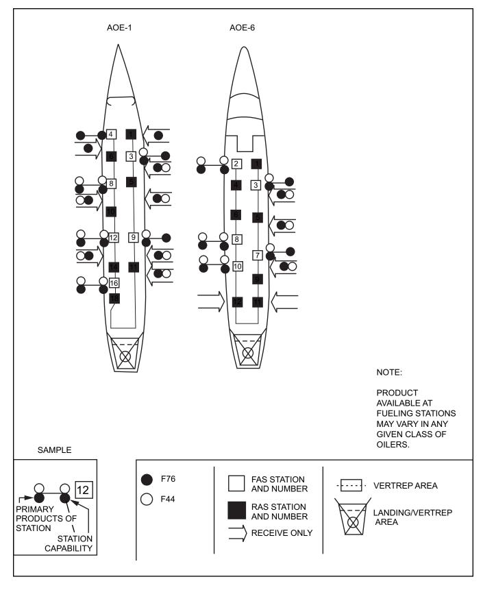
Figure 3-2. Typical Transfer Stations on Oilers (Sheet 1 of 2)
