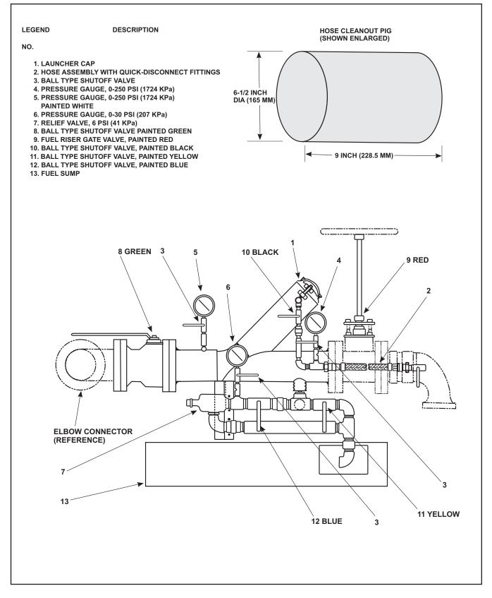
Figure 5-10. Pig Launcher Assembly and Hose Cleanout Pig
