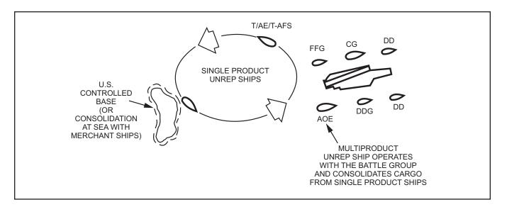
Figure 1-1. U.S. Navy Underway Replenishment Concept
