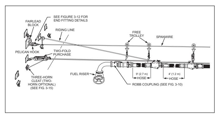
Figure 4-2. Securing the Single Hose With Robb Coupling
