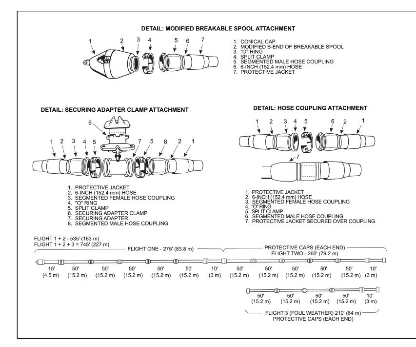
Figure 5-11. Astern Refueling Hose Assembly (Merchant Tanker)
