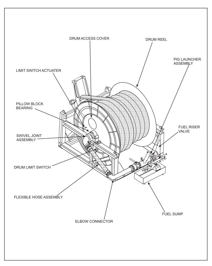
Figure 5-4. Astern Refueling Hose Reel Assembly (View B)
