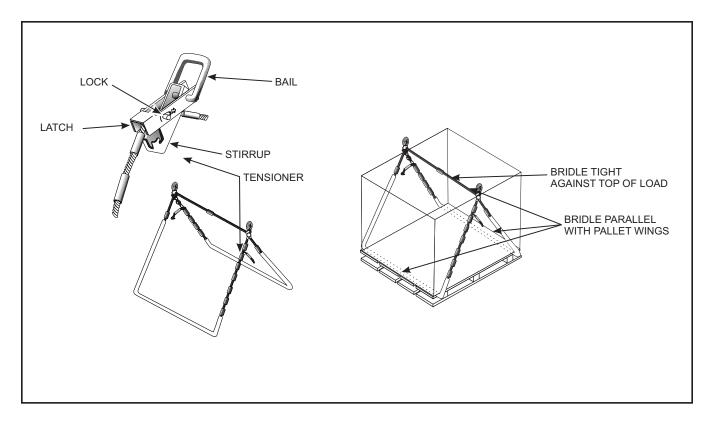
Figure 10-6. Adjustable Pallet Sling
