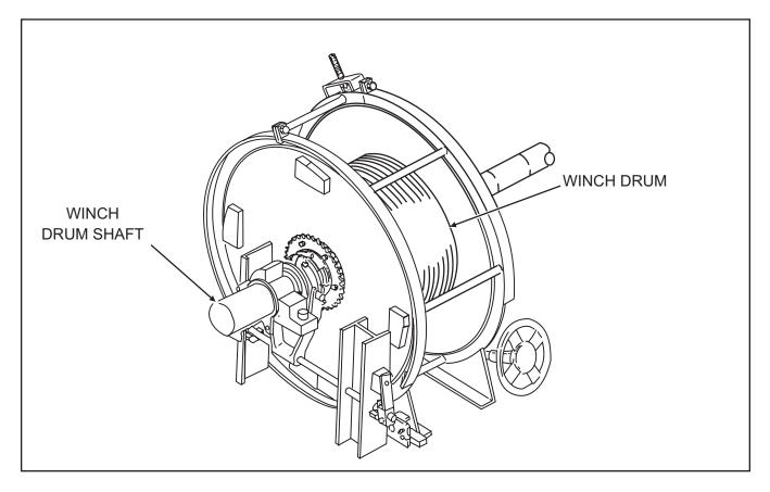
Figure 8-6. Typical Inhaul Winch Drum Without Slip Clutch
