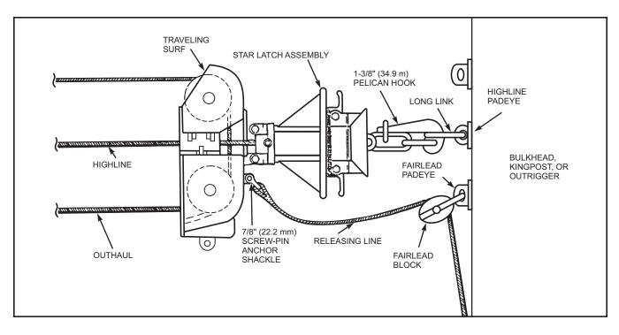
Figure 6-13. Fixed Padeye Receiving Station (Typical) — Shown With STREAM With STAR
