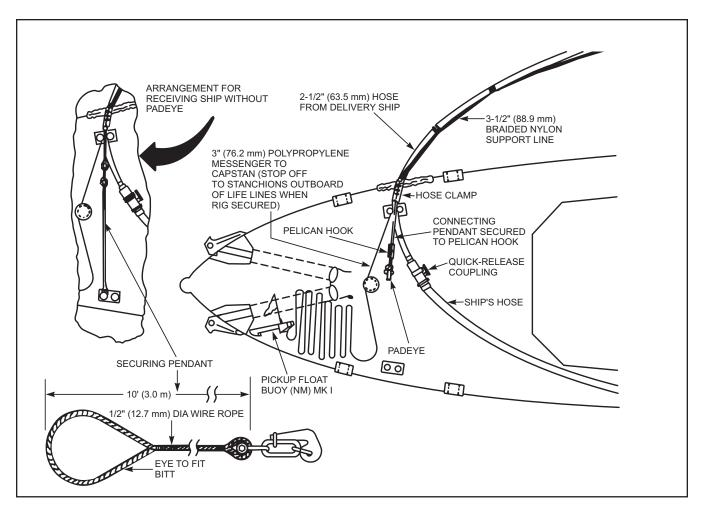
Figure 5-24. Streaming Astern Fueling 2-1/2-Inch (63.5 mm) Hose (Sheet 2 of 2)
