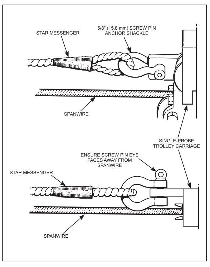
Figure 3-25. Attachment of STAR Messenger Shackle to Trolley Carriage
