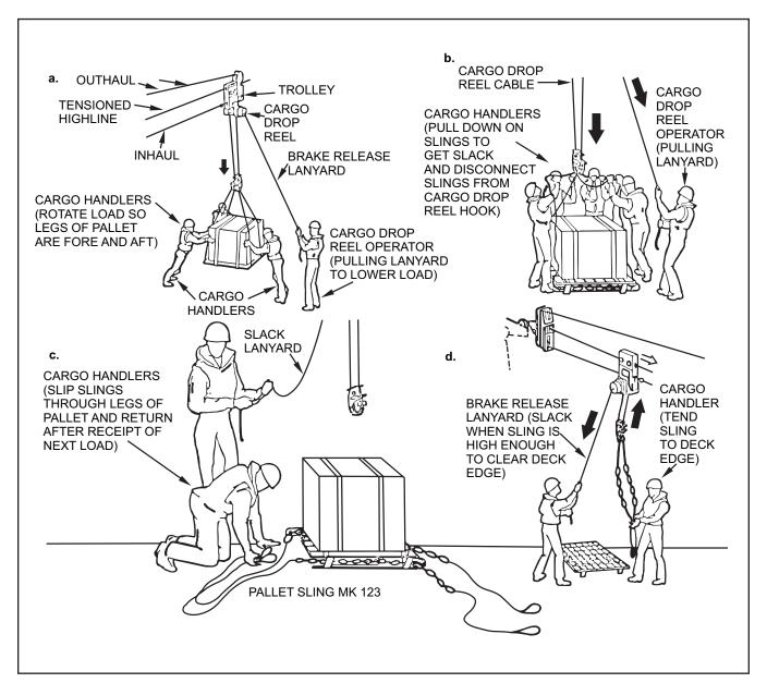
Figure 6-33. Handling Palletized Ammunition
