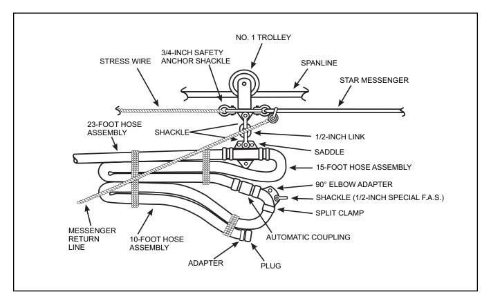
Figure 4-8. Nontensioned Spanline Fuel Rig at Trolley No. 1
