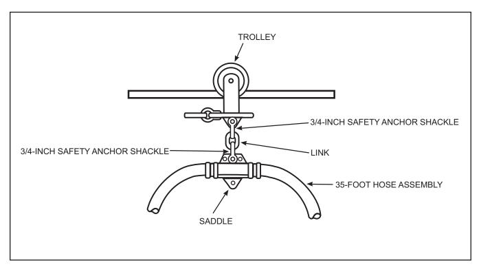
Figure 4-7. Nontensioned Spanline Fuel Rig at Trolley Nos. 2 and 3
