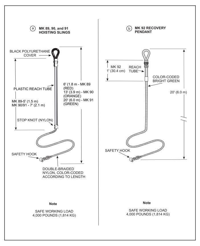
Figure 10-9. Hoisting Sling Mk 89, 90, and 91 (Single-Leg) and Recovery Pendant Mk 92
