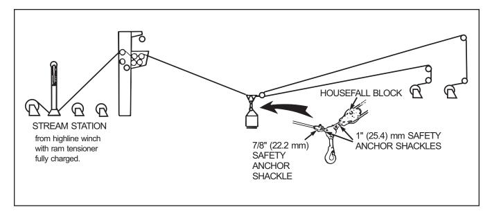
Figure 7-7. Basic Heavy-Lift/Double-Whip Burton Configurations
