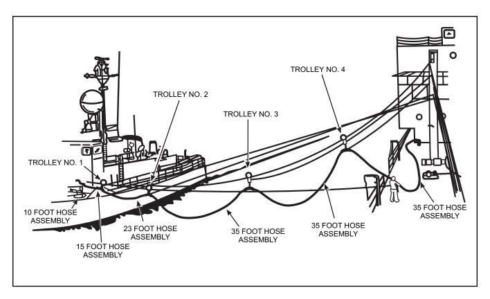
Figure 4-5. Nontensioned Spanline Fuel Rig (188 Feet)
