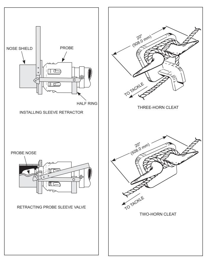
Figure 3-16. Probe Sleeve Retractor
