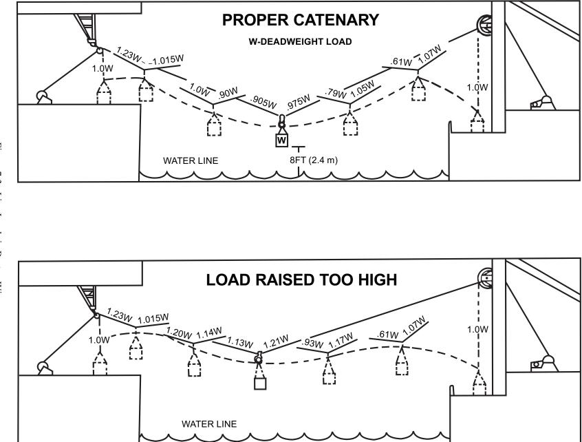
Figure 7-3. Line Loads in Burton Wires
