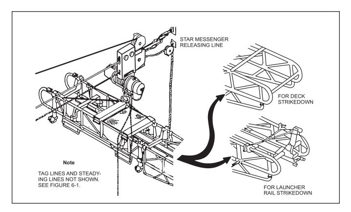
Figure 6-9. Cargo Drop Reel With Mk 6 Dolly
