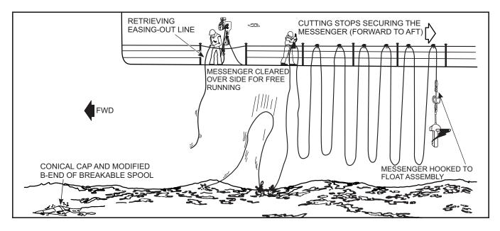
Figure 5-21. Hose Messenger Rigged for Disengaging
