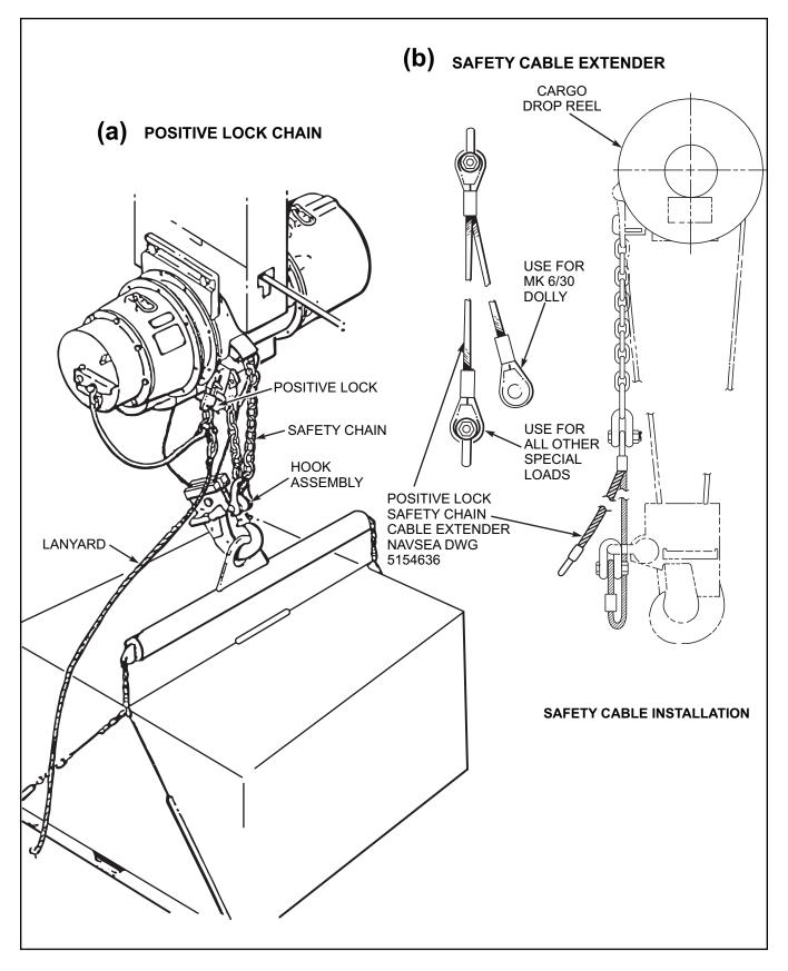
Figure 6-10. Positive Lock Safety Chain and Cable Extender
