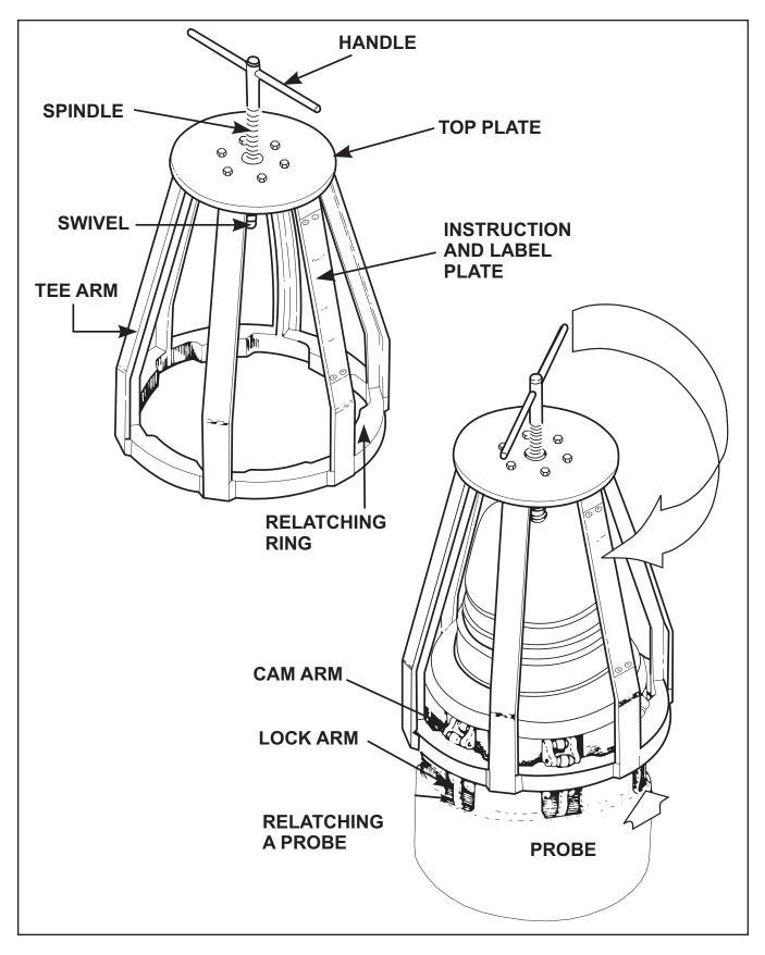
Figure 3-15. Probe Relatching Tool
