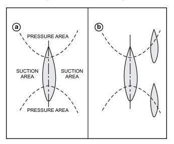
Figure 2-4. Dangers of Hull Wash
