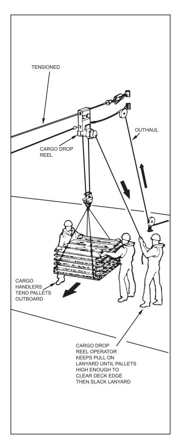
Figure 6-32. Returning Empty Pellets
