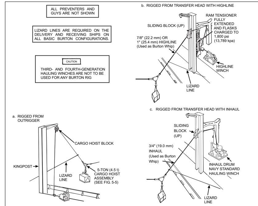
Figure 7-4. **Basic Burton Configurations**
