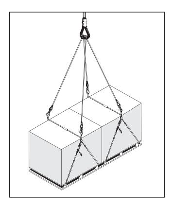
Figure 10-16. Hoisting Sling Mk 105 With Two-Pallet Load (Four Attachment Points)
