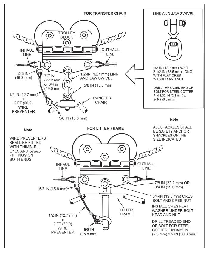
Figure 9-2. Rigging the Trolley for Personnel Transfer
