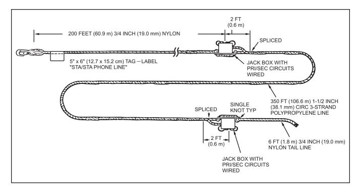
Figure 2-13. Station-to-Station (Sta/Sta) Phone Line
