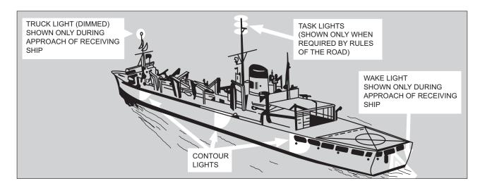
Figure 2-17. Approach and Station-Keeping Lights
