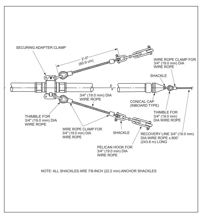
Figure 5-5. Hose Securing Pendant and Adapter
