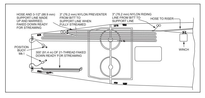
Figure 5-22. Typical Astern Fueling Station Keeping With 2-1/2-Inch (63.5 mm) Hose
