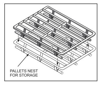
Figure 10-2. Nestable Tubular Steel Pallet
