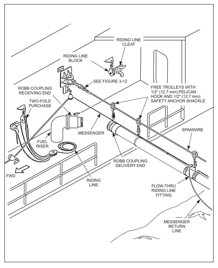
Figure 3-24. Single-Hose Fuel STREAM Rig With Robb Coupling
