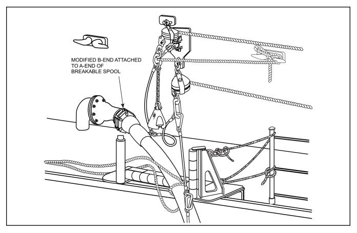
Figure 5-19. Receiving Station Rigged for Fuel Transfer
