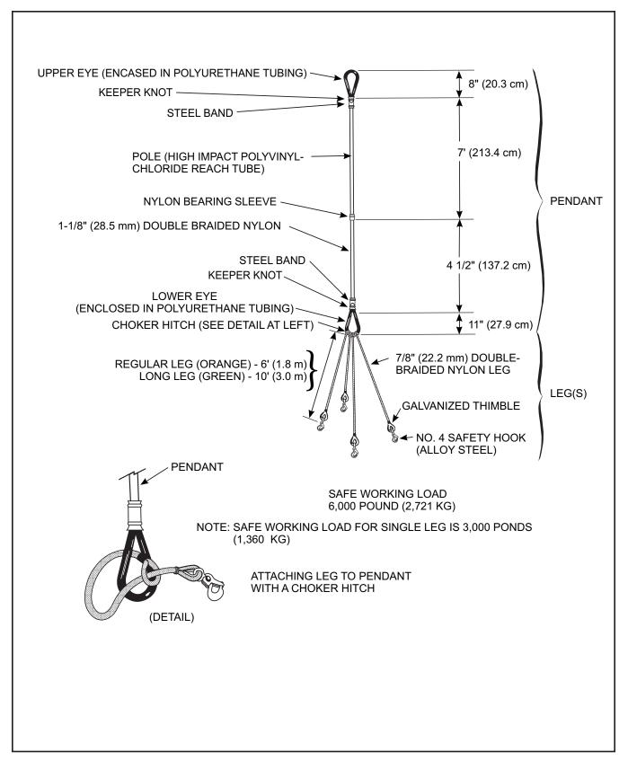
Figure 10-8. Mk 105 Hoisting Sling (Multileg-Pole Pendant)
