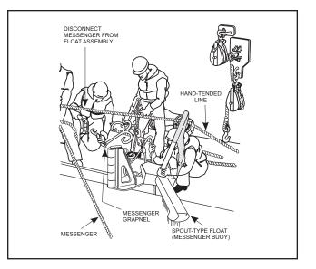
Figure 5-15. Disconnecting the Hose Messenger
