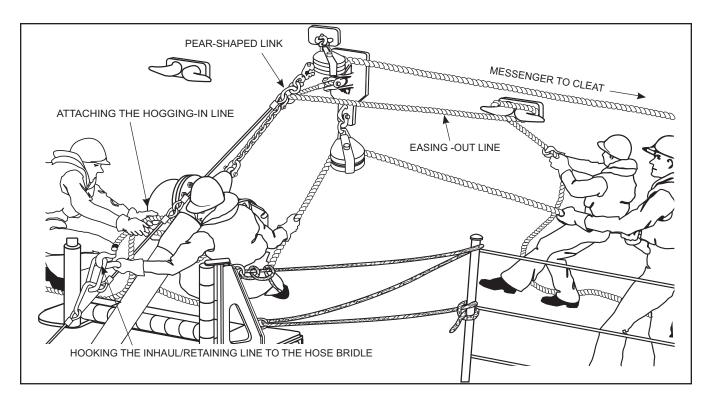
Figure 5-16. Securing the Hose Rig
