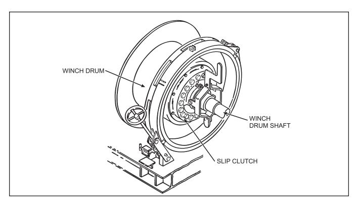
Figure 8-5. Typical Fourth Generation Inhaul Winch Drum With Slip Clutch
