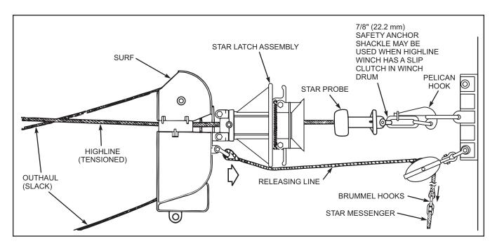
Figure 6-21. STREAM With STAR for Highline With Slip Clutch in Drum — Haul Into Receiving Station
