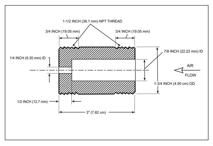
Figure J-2. Orifice for Blowdown Air Line
