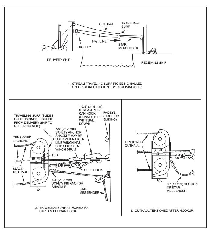
Figure 6-23. STREAM With Traveling SURF — Rigging at the Receiving Station
