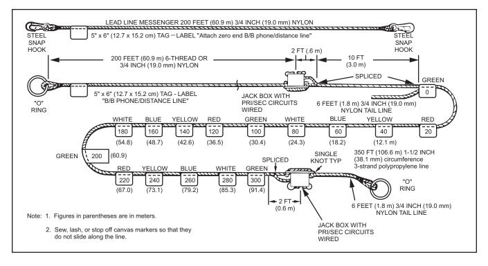
Figure 2-10. Bridge-to-Bridge (B/B) Phone/Distance Line
