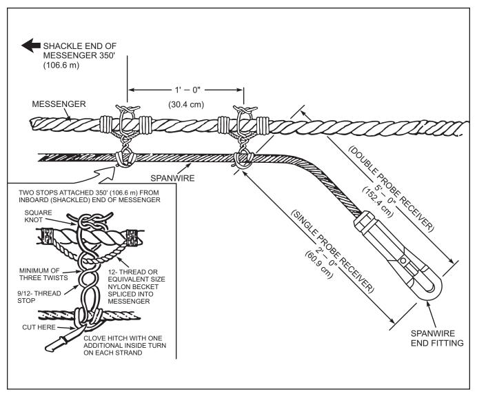
Figure 3-21. Method of Stopping the Span Wire to the Messenger
