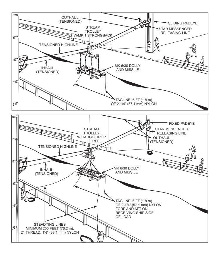
Figure 6-8. Missile Transfer in Mk 6 Dolly To Sliding Padeye (Upper) or to Fixed Padeye (Lower)
