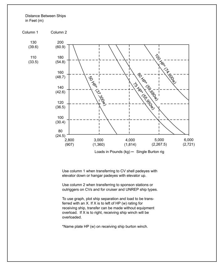
Figure 7-2. Maximum Transfer Loads for Single-Burton Rig Without Winch Overload
