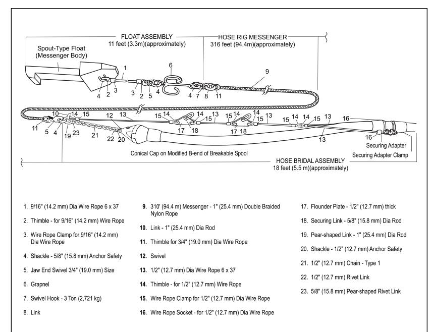
Figure 5-7. Float Assembly, Hose Messenger, and Hose Bridle Assembly
