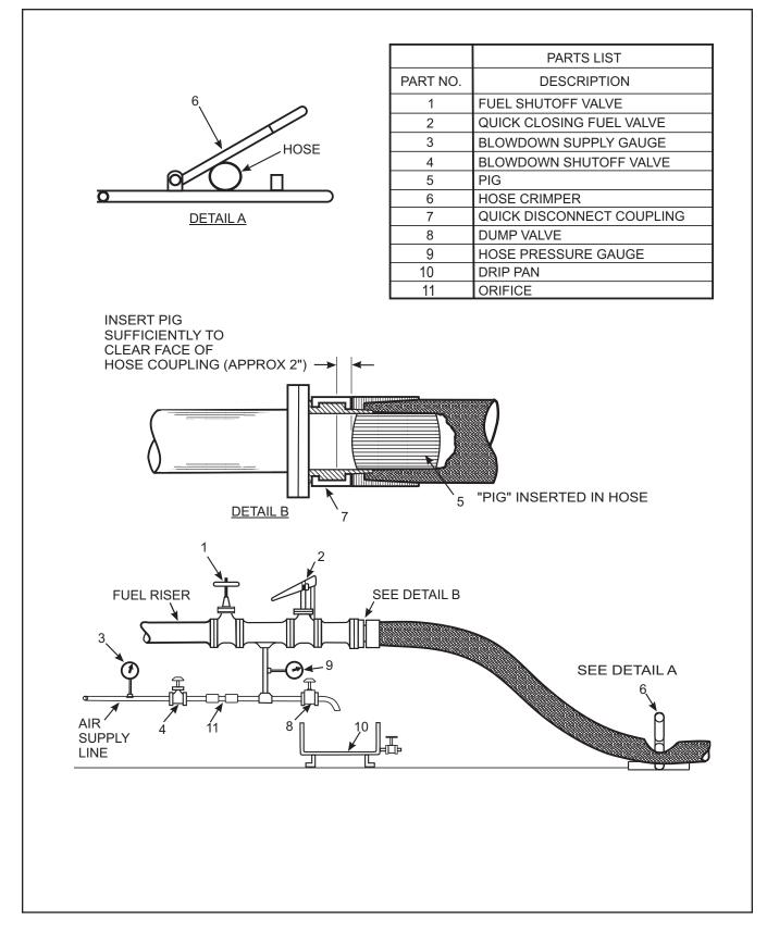
Figure J-3. Astern Refueling Station — Delivery Ship
