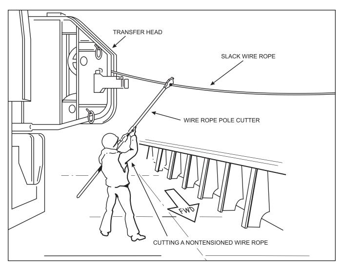
Figure 2-5. Cutting a Nontensioned Wire Rope
