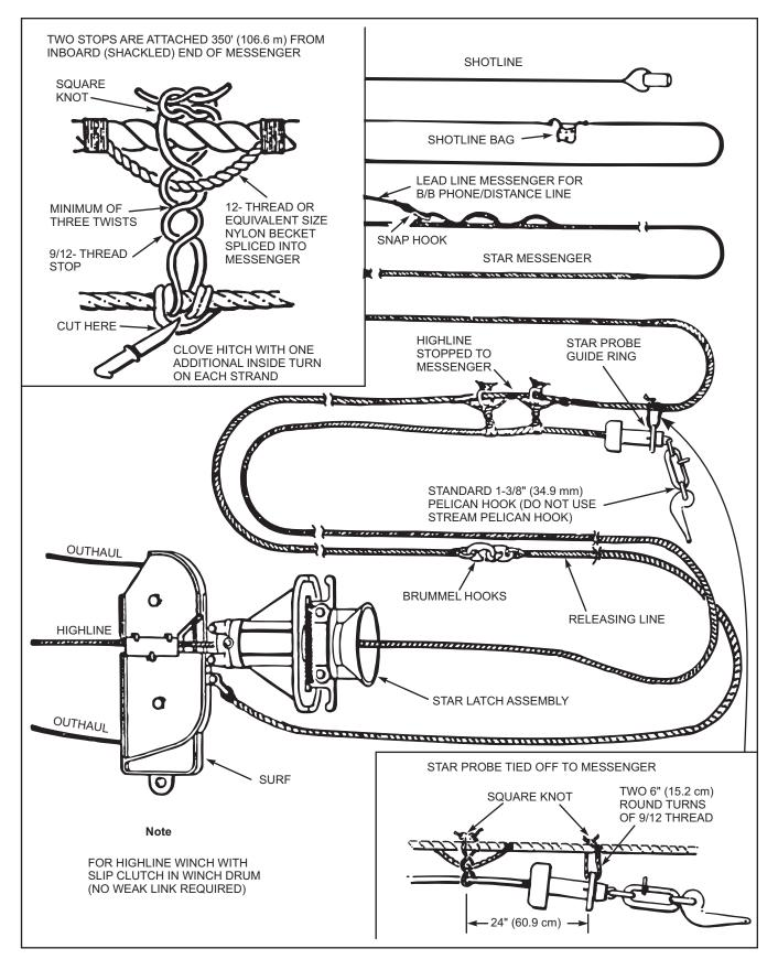
Figure 6-19. STREAM With STAR — Rig Layout at the Delivery Station (Sheet 2 of 2)
