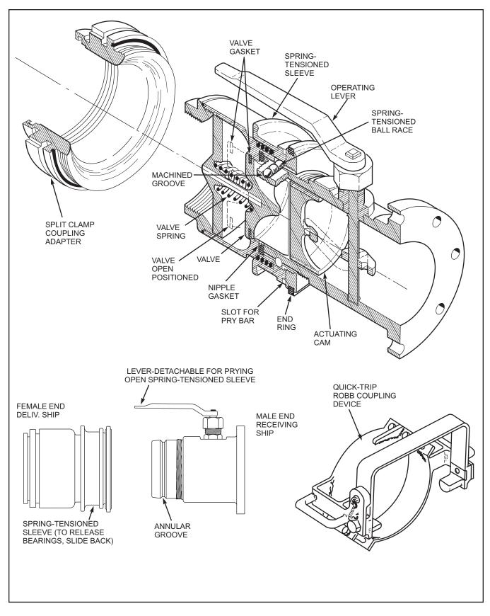
Figure 3-11. Combined Quick-Release Coupling and Valve (Robb Coupling)
