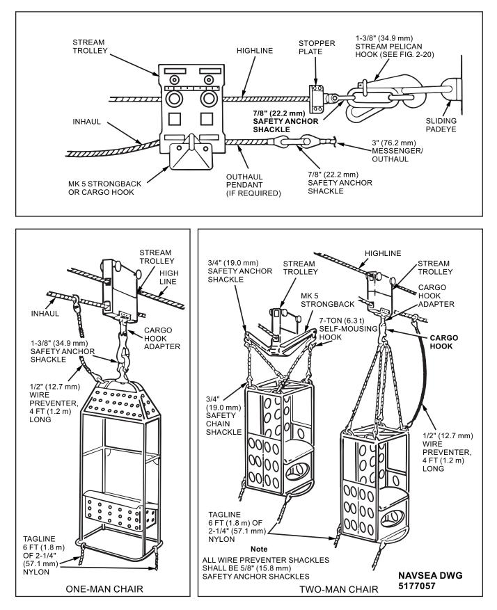
Figure 8-2. Personnel STREAM — Rigging Details for Transfer to Sliding-Padeye or Sliding-Block Receiving Station
