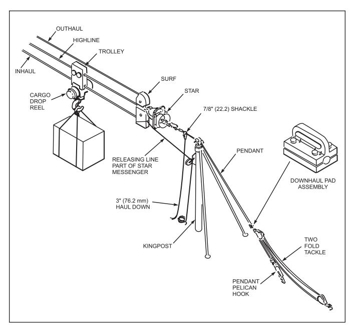
Figure 6-14. Pendant Receiving Station (Typical) — Shown With STREAM With STAR
