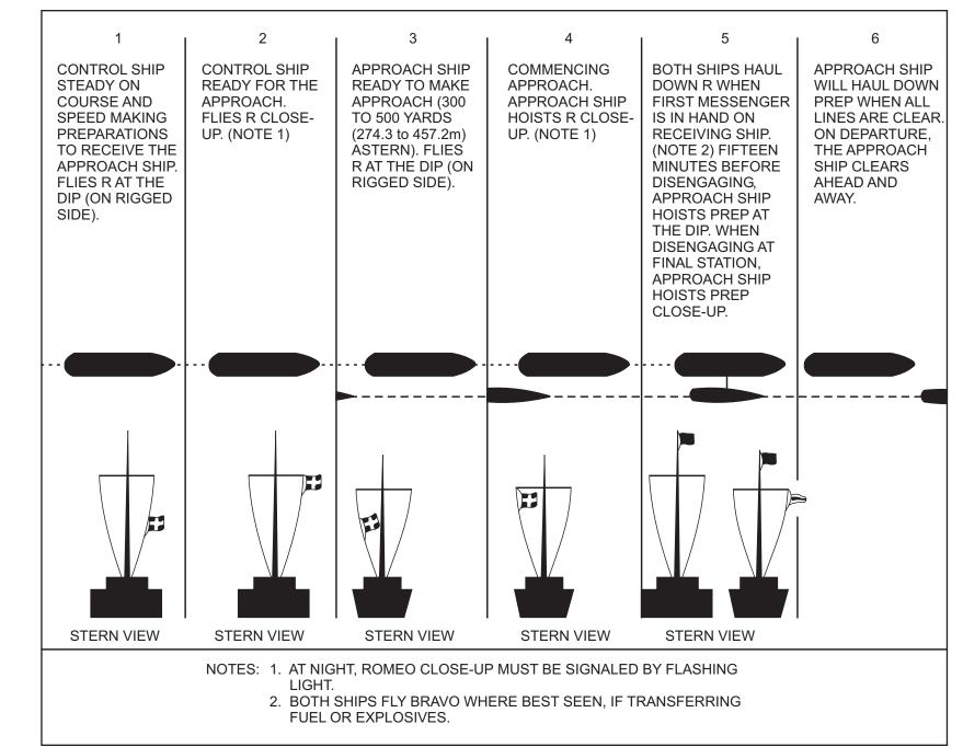
Figure 2-2. Flag Hoist Procedure Approach, Riding Alongside, and Departure
