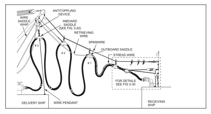
Figure 4-1. Nontensioned Spanwire Fuel Rig (Signle Hose With Robb Coupling)
