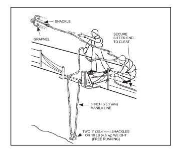
Figure 5-14. Heaving the Grapnel Line
