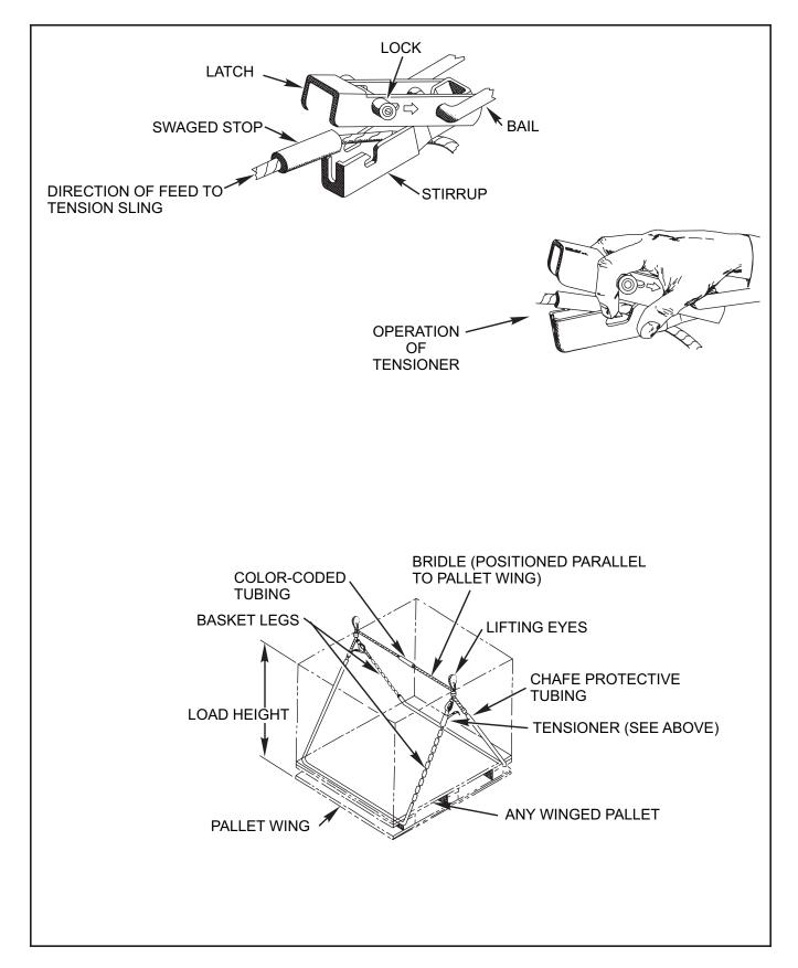
Figure 10-14. Adjustable Pallet Sling Mk 85, 86, 87, and 100
