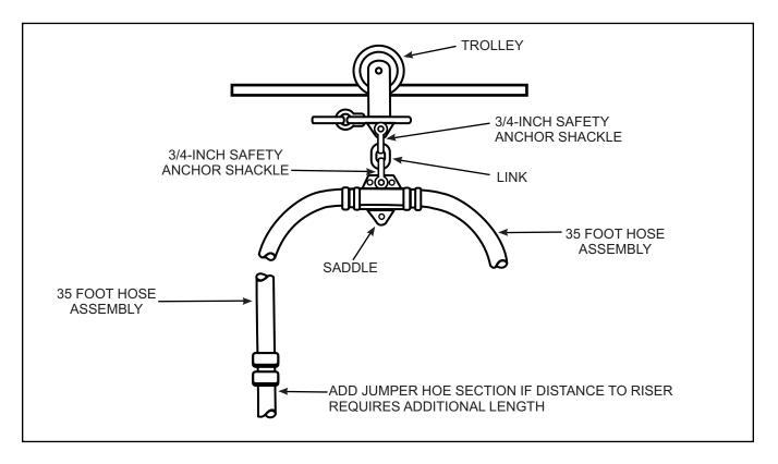
Figure 4-6. Nontensioned Spanline Fuel Rig at Trolley No. 4
