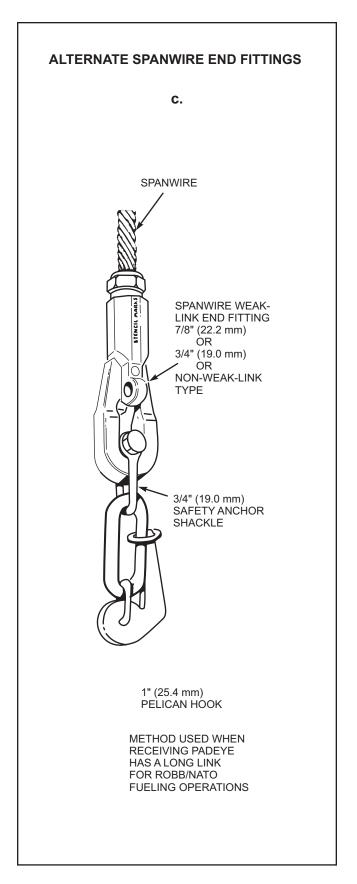
Figure 3-14. Spanwire End Fittings for Fueling Rigs (Sheet 2 of 2)
