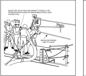
Figure 5-17. Disconnecting the Conical Cap
