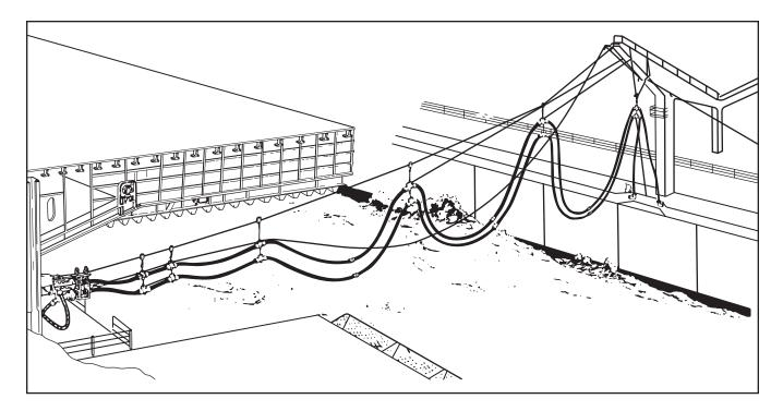
Figure 3-29. Double-Hose Fuel STREAM Rig (With Double Probe)
