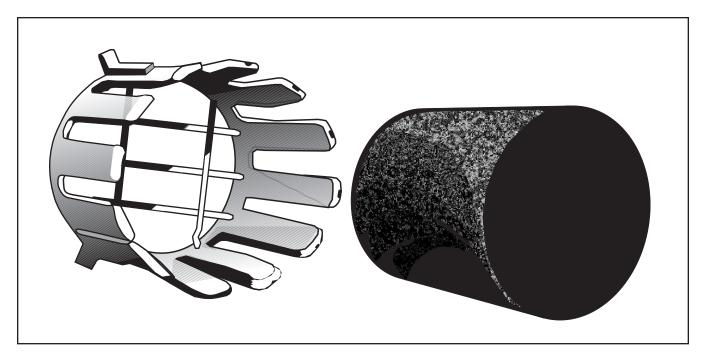
Figure J-1. Pig Catcher (Left) and Pig (Right)
