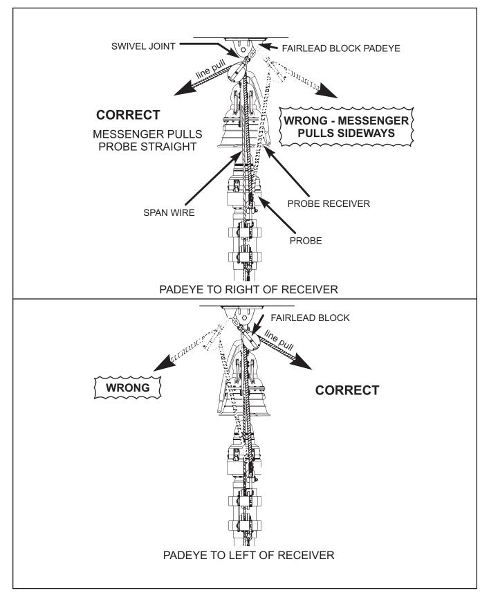
Figure 3-26. Messenger Fairlead at Receiving Station (Top View)
