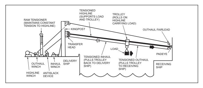
Figure 6-2. STREAM Rig (All Tensioned Wires)
