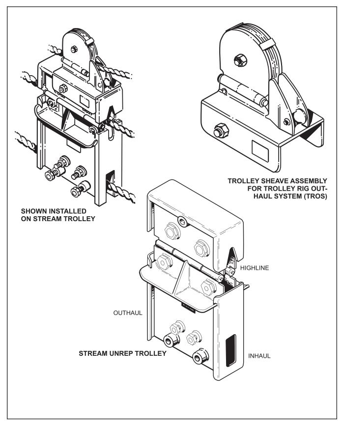
Figure 6-7. STREAM Trolleys
