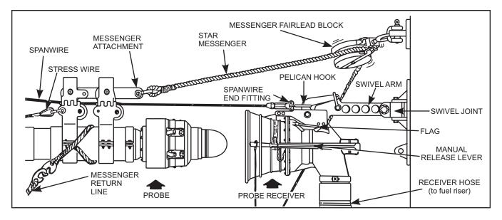
Figure 3-23. Single-Hose Fuel STREAM Rig With Probe
