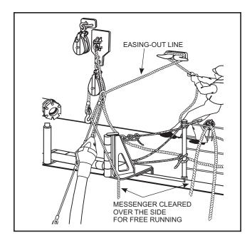
Figure 5-20. Easing the Hose Overboard
