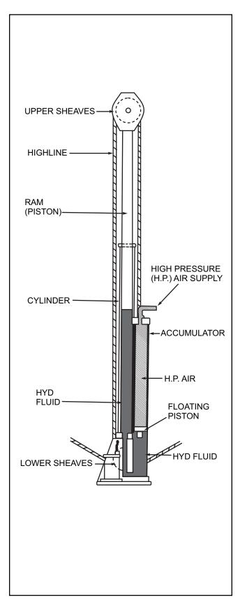
Figure 6-3. Ram Tensioner (Cross-Section)
