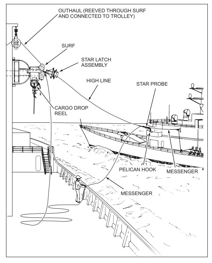
Figure 6-20. STREAM With STAR — Passing the Rig
