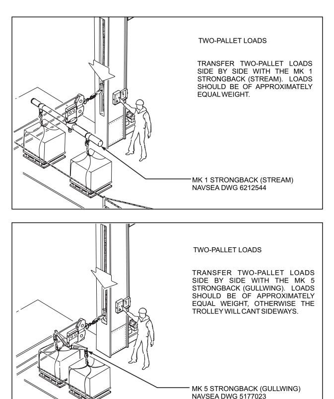
Figure 6-12. Sliding-Padeye Receiving Station (Typical) — Shown With STREAM With Traveling SURF (Sheet 2 of 2)
