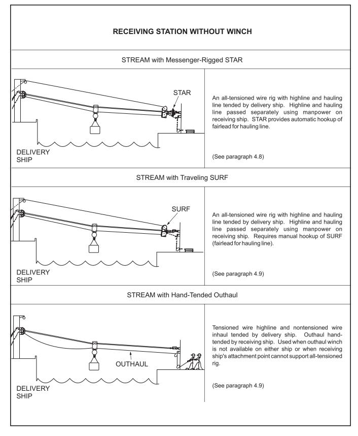
Figure 6-15. STREAM Rig Configurations
