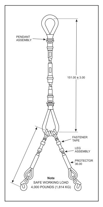
Figure 10-10. Pendant Assembly — Hoisting Sling Mk 128 Mod 0
