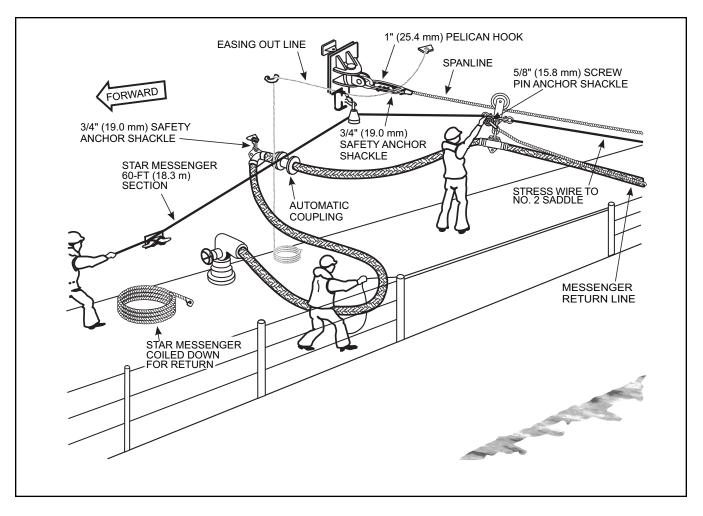
Figure 4-9. Receiving the Nontensioned Spanline Fuel Rig
