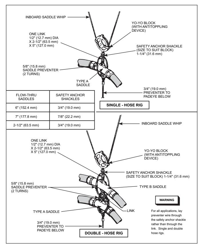
Figure 3-22. Inboard Saddle Arrangement
