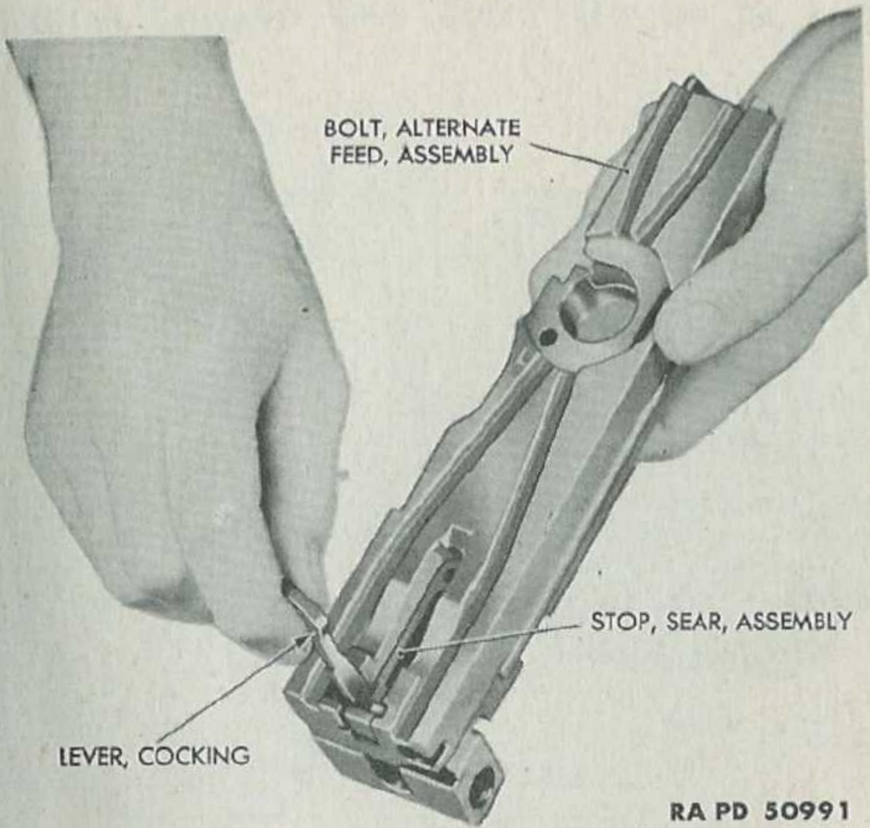
Figure 37—Disengaging Sear Stop Assembly
