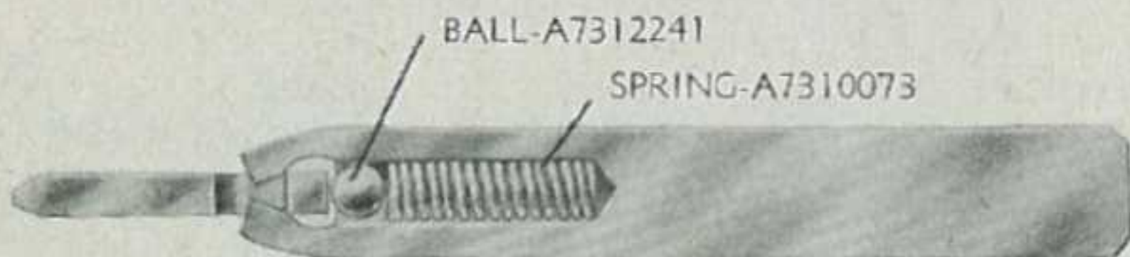
Figure 78—Removing Trigger Bar Pin Assembly (Old Type)
