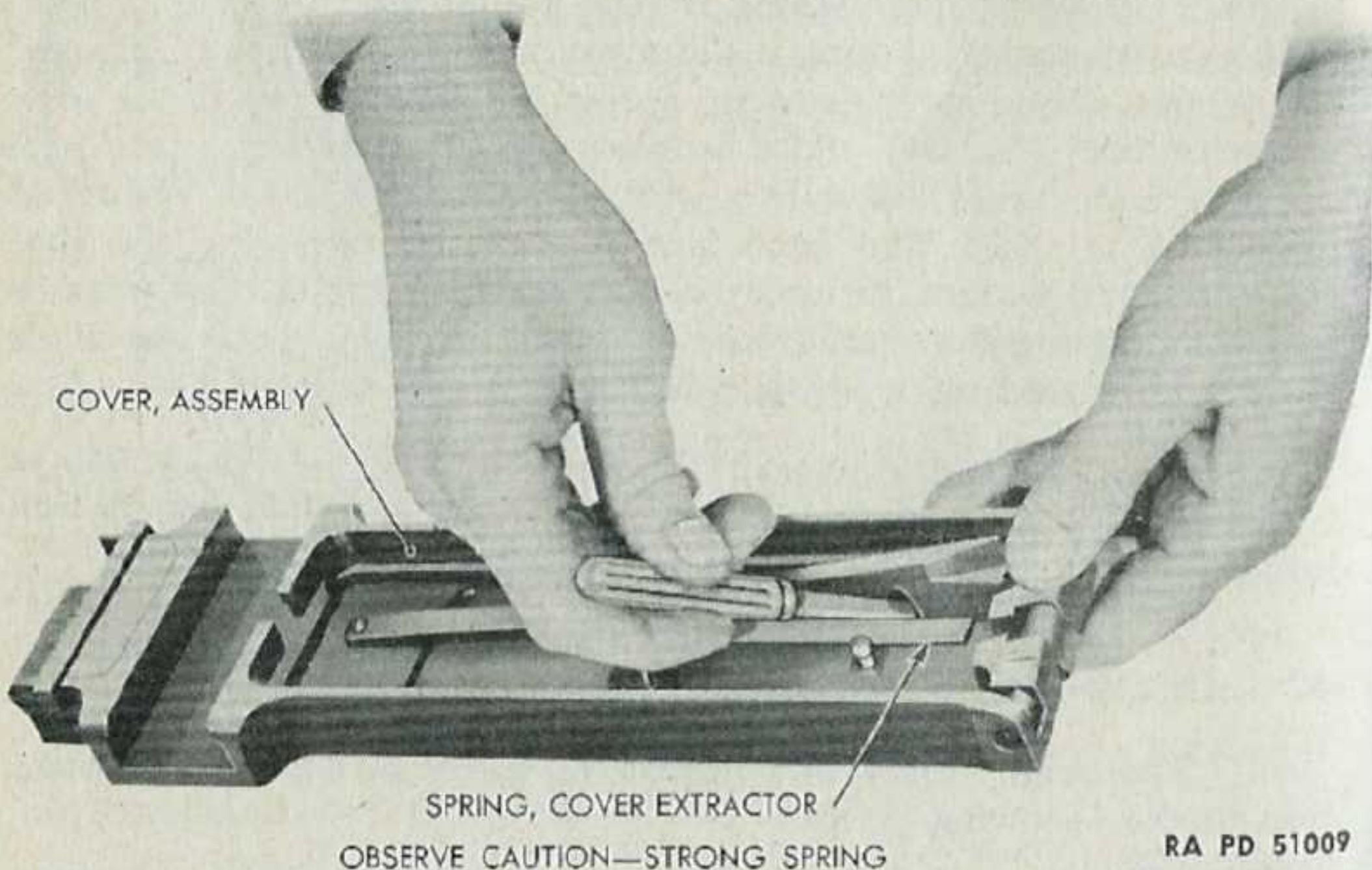
Figure 64—Removing Cover Extractor Spring
