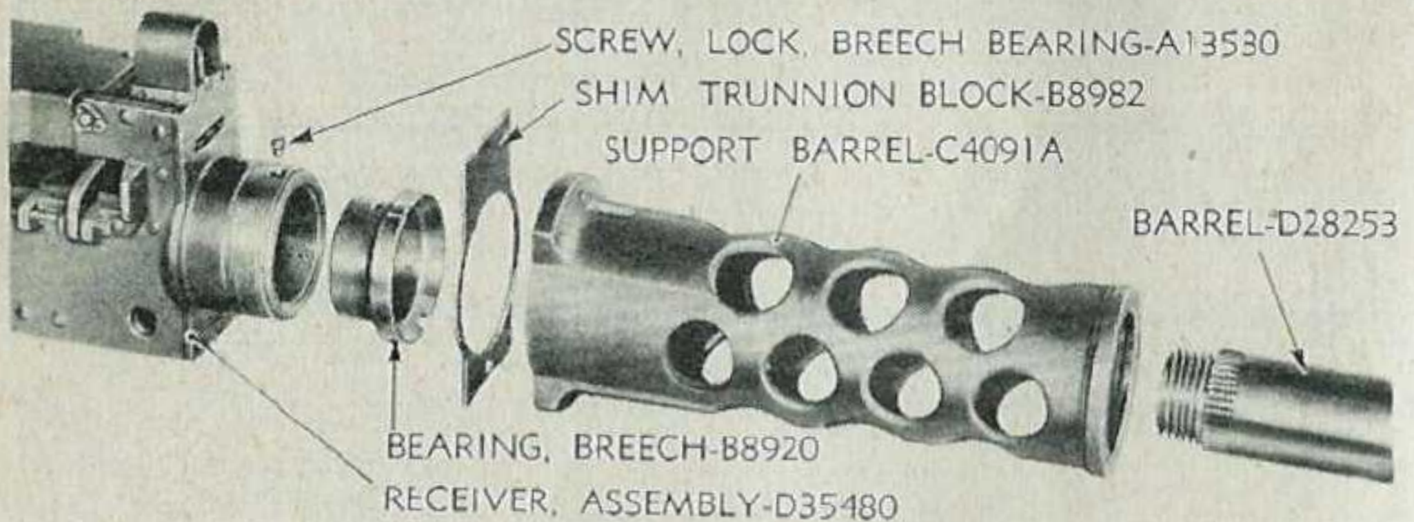
Figure 86—Water Jacket Removed From Receiver
