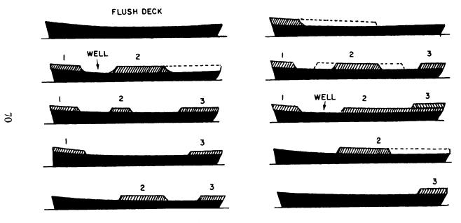
Figure 28.—Basic hull designs.
