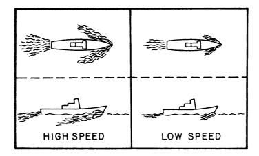
Figure 13.—Bow wave and stern wake.
