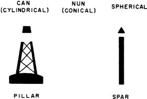
Figure 23.—Basic buoy shapes.
