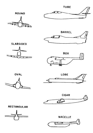
Figure 32.—Fuselage types.
