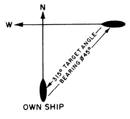
Figure 10.—Target angle.
