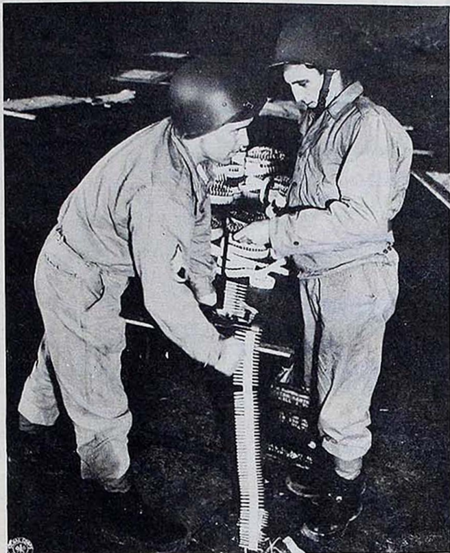
FIGURE 144—BELTING CALIBER .30 MACHINE GUN AMMUNITION IN THE FIELD
