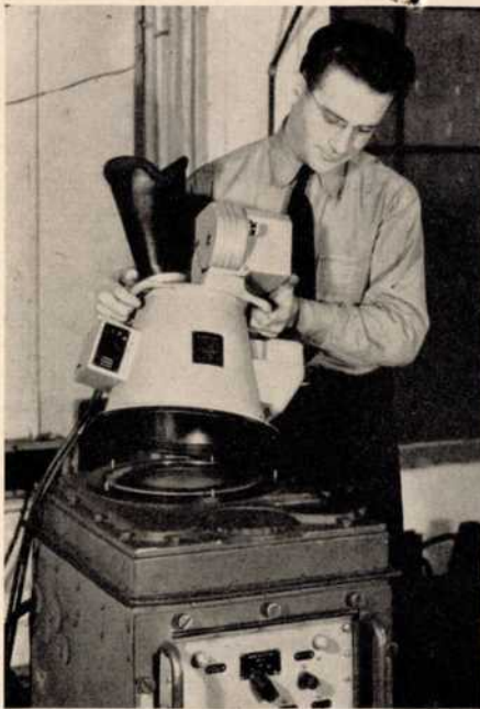
■ The mounting of the camera on a PPI scope is a simple process, accomplished in slightly less than jig time.
