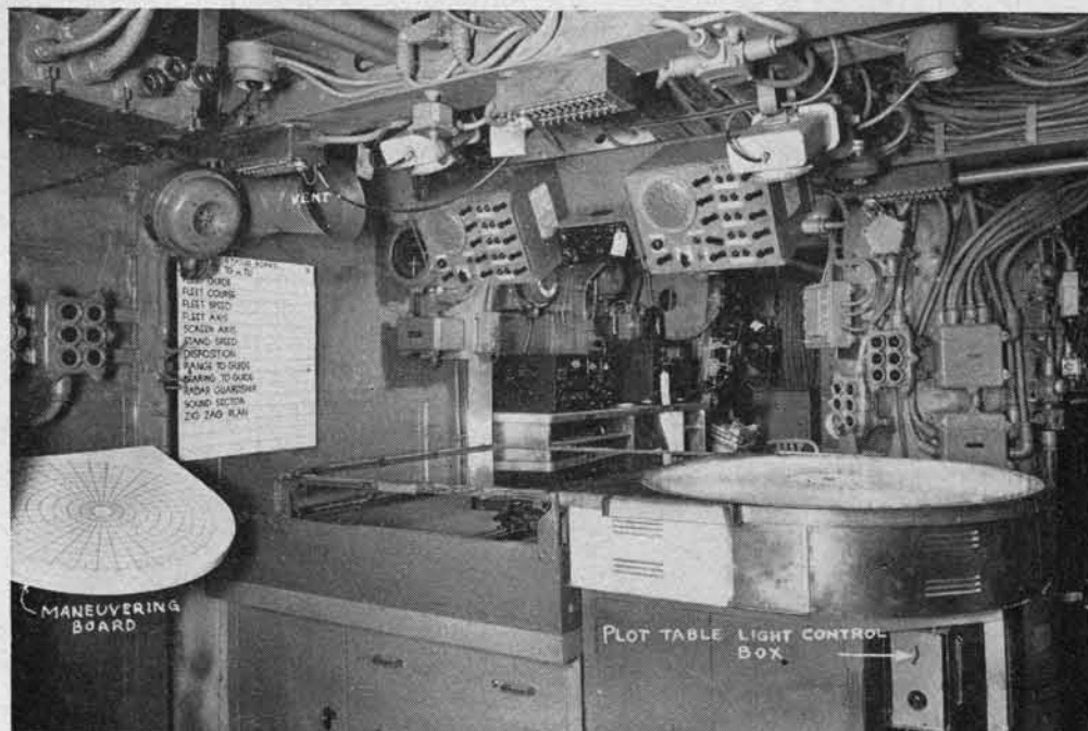
CL (6,500 tons), showing evaluator's position. This CIC contains (next to far right-hand corner of DRT) a chemical recorder from which the range rate of submarines may be determined, and the sound stack (behind the fire-control tube) giving range and bearing of submarines. Note the convenient location of the battle hand lanterns bolted to the overhead. The maneuvering board beside the DRT and Plot Table is an unusual feature.
