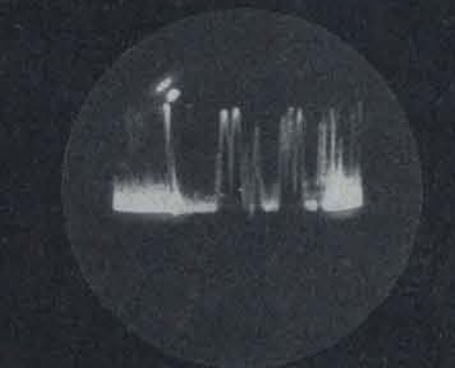
7 FD C and I: Window appearance on FD scope. There are no targets here besides Window.
