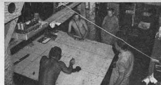
AWS-1 CIC interior snapped while a lost B-24 was being homed. Note VHF loudspeaker above beam at left.
